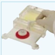
NEW-style Flexicasters allow the casting of varying gel lengths simply by locking the moveable dam. Adjustable feet and level bubble allow gels of uniform thickness to be poured.
