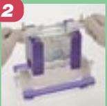
Transfer to casting base and tighten cams
