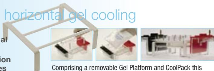
Comprising a removable Gel Platform and CoolPack this unique system will cool the buffer chamber of multiSUB horizontal gel units without any external chilling. Simply place the platform over the running tray and place a pre-chilled CoolPack on top. This allows the CoolPack to sit above the gel in buffer directly removing any heat generated.
