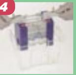
Transfer to tank, fill with buffer and run
