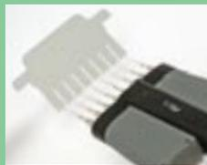
The number of samples can be maximised using high tooth number combs
