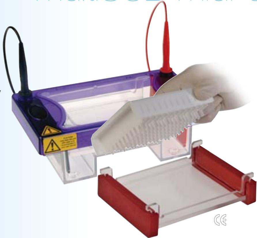
**Ideal for analysis of up to 96 PCR-fragment length polymorphisms loaded from 96-well microplates or thermal cycler blocks**
